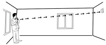
5. The DRC range calculated by the detector will be displayed as a number of pulses from 1 to 3.
