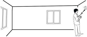
4. Go to the furthest distance (max. 9 m) of the glass to be protected and aim the speaker at the detector.
