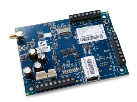
With the IRIS-4 6series, AddSecure offers a cost-effective bus integration terminal for alarm panels of leading manufacturers.
