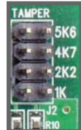
\*The KX15DTAM also has Mask / Fault Selectable EOL resistors.
